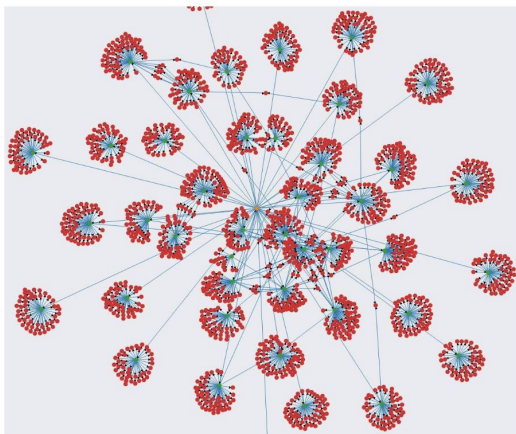
Figure 2: Visualization of the level-2 social graph for a single “target” account in DEC. The centered orange node is the target node to classify. The blue nodes are the neighboring nodes from the first fan-out level. The red nodes are from the second fan-out level. An edge between two nodes represents the relation of mutual friends. For each node visualized in this graph, hundreds of features are extracted and aggregated for classification.
